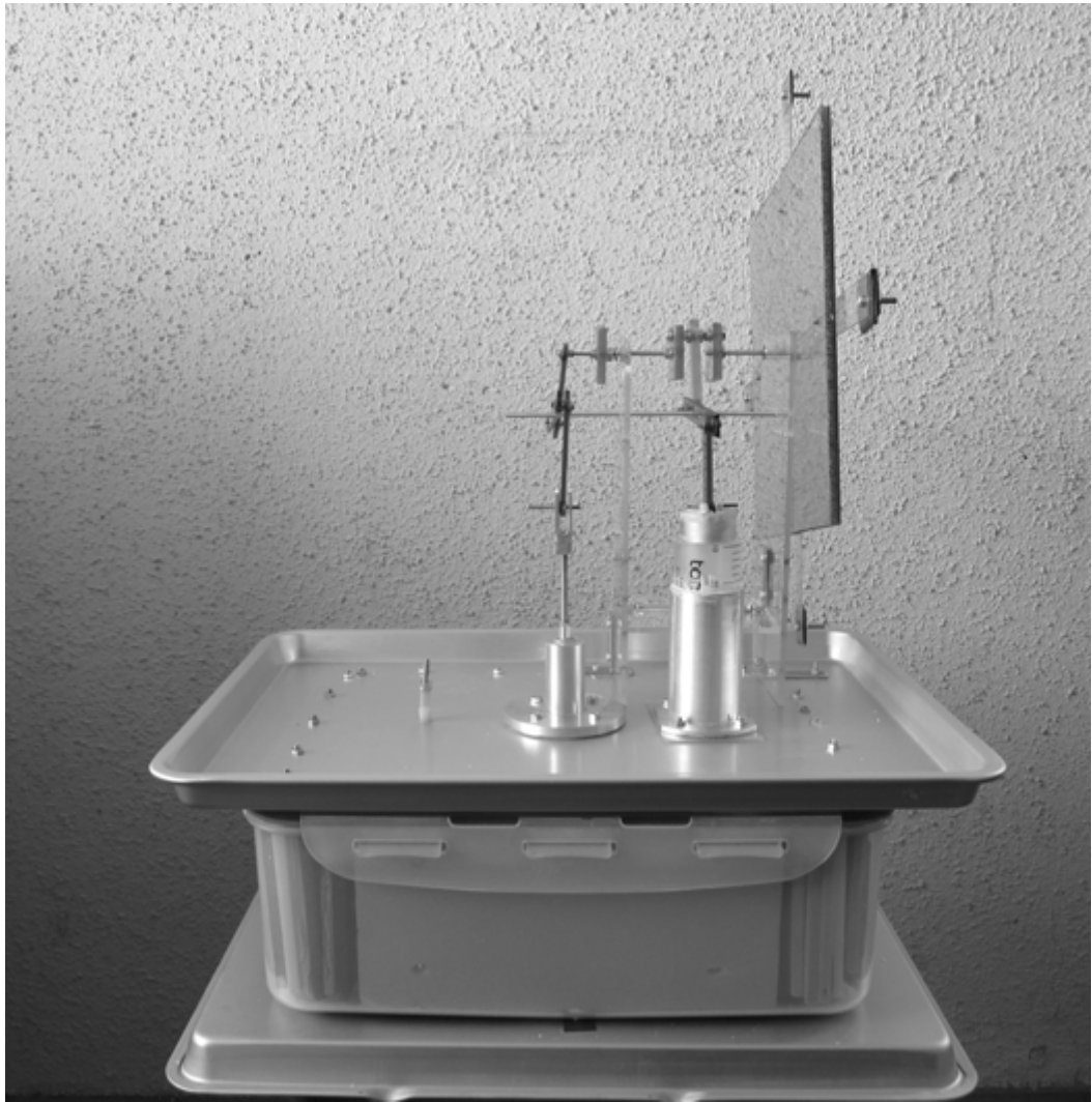
Fig.4-1 Structure of testing LTD stirling engine
