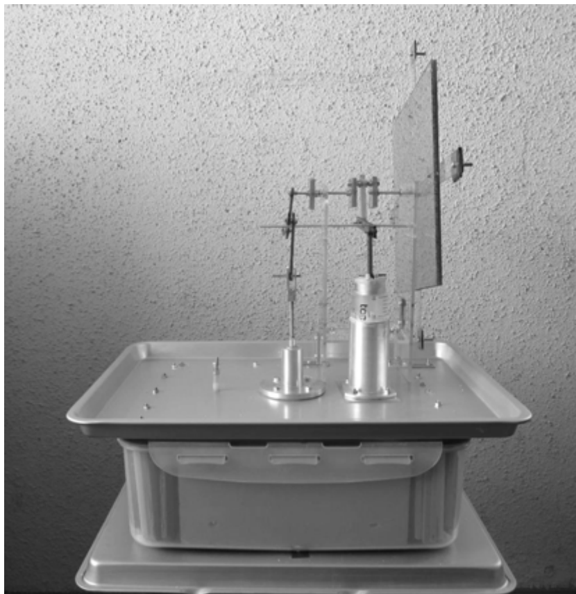
Fig.A14 Structure of low temperature testing stirling engine
